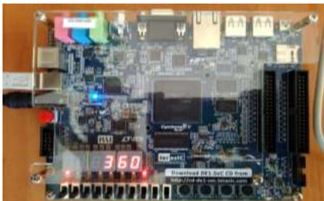
Figure 4 — DE1-SoC Development Kit with Cyclone V FPGA during hardware verification of designed controller
