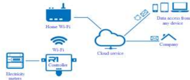
Figure 2 — The principle of remote collection of readings from an electricity meter
