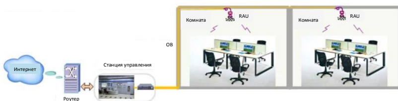
Picture 2 – WiFi-RoF network architecture for internal localization
