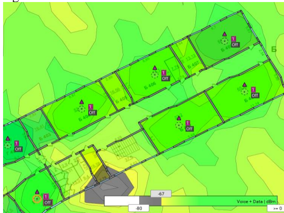
Figure 6 – Simulation results for compartment B in the 2.4 GHz band with increased placement of access points in classrooms
