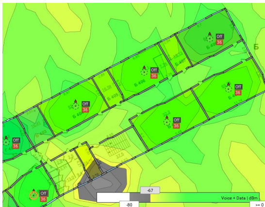
Figure 6 – Simulation results for compartment B in the 2.4 GHz band with increased placement of access points in classrooms
