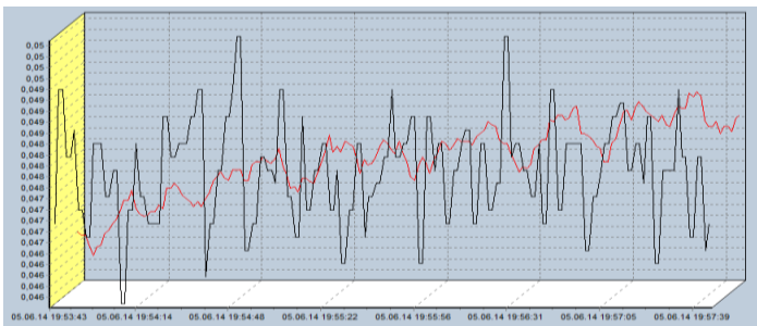
Figure 2 – Shot-time temperature measurement non-stability in the melting ice among the sensors of metrological class \pm 0,03^{\circ}\text{C}
