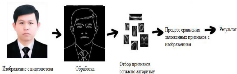
Figure 3 — The process of facial recognition using neural networks compiled in Python
